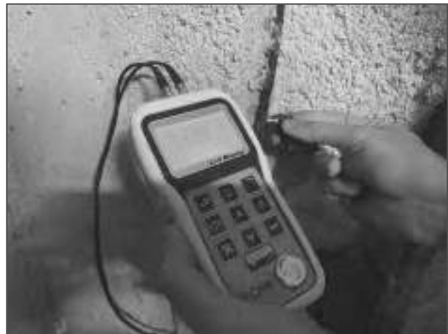
Photograph 9 – UTG reading of the flange thickness on the lower part, 2 nd reading.
