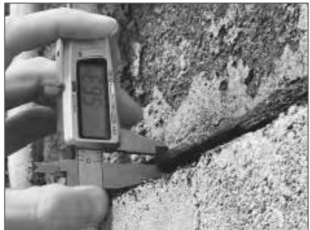
Photograph 17 – remaining thickness of the beam flange, 2 nd reading
