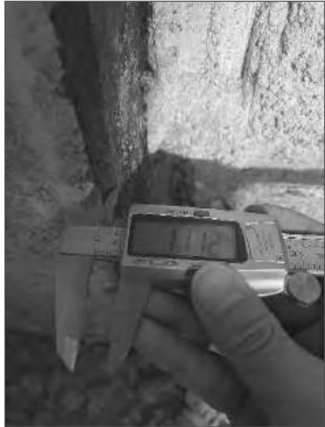
Photograph 11 – calibrator estimation, confirmation of the thickness
