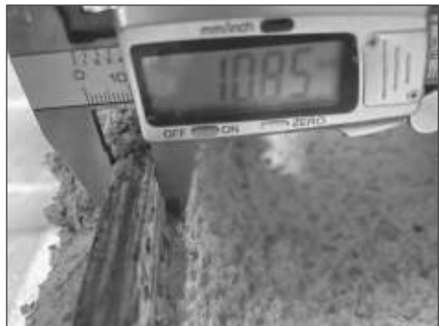
Photograph 6 – calibrator representing the flange thickness on the upper part by calibrator
