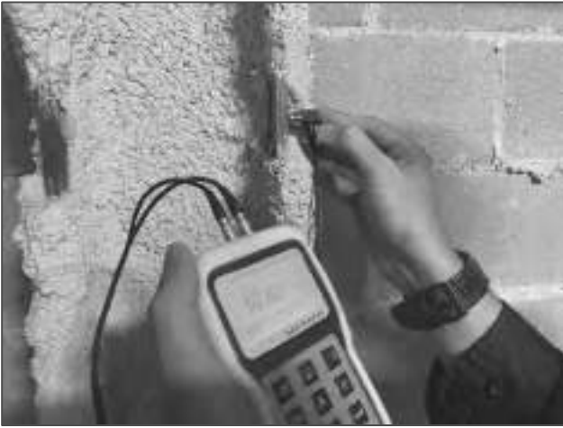
Photograph 7 – UTG readings on flange of upper area
