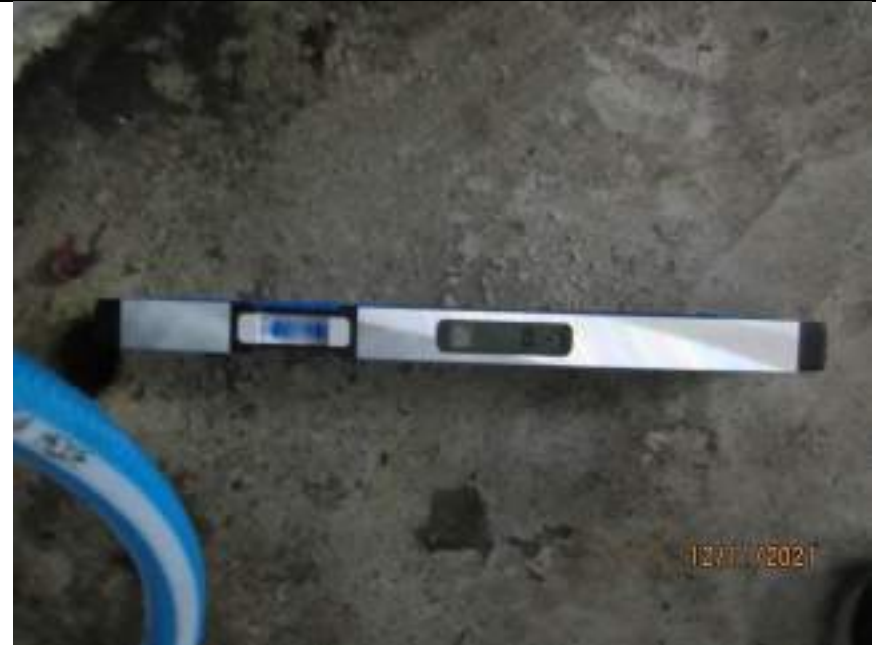
Zero fall indicated to eastern side of drainage inlet
