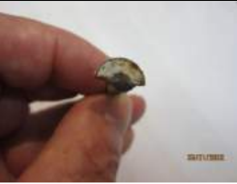
Evidence of corrosion to metal screws used to fix battens found with demolition waste located in Basement 2 storage area
