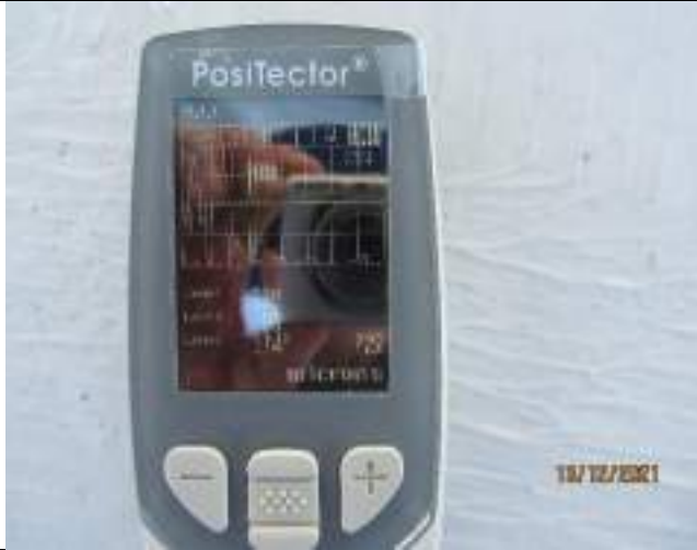
Test indicating 722 micron thickness
